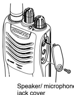
If you are not using a speaker/ microphone, install the cover over the speaker/ microphone jacks using the supplied M3 x 6 mm screw.
